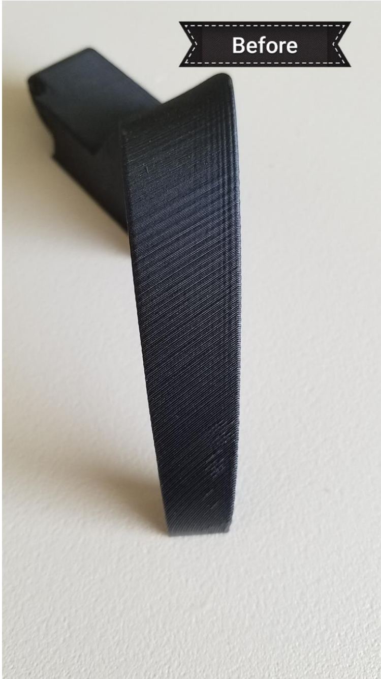
Pic 1f Your claws have layer lines from the 3D printing process. In the following steps we will go from this to a smooth surface ready for paint.
