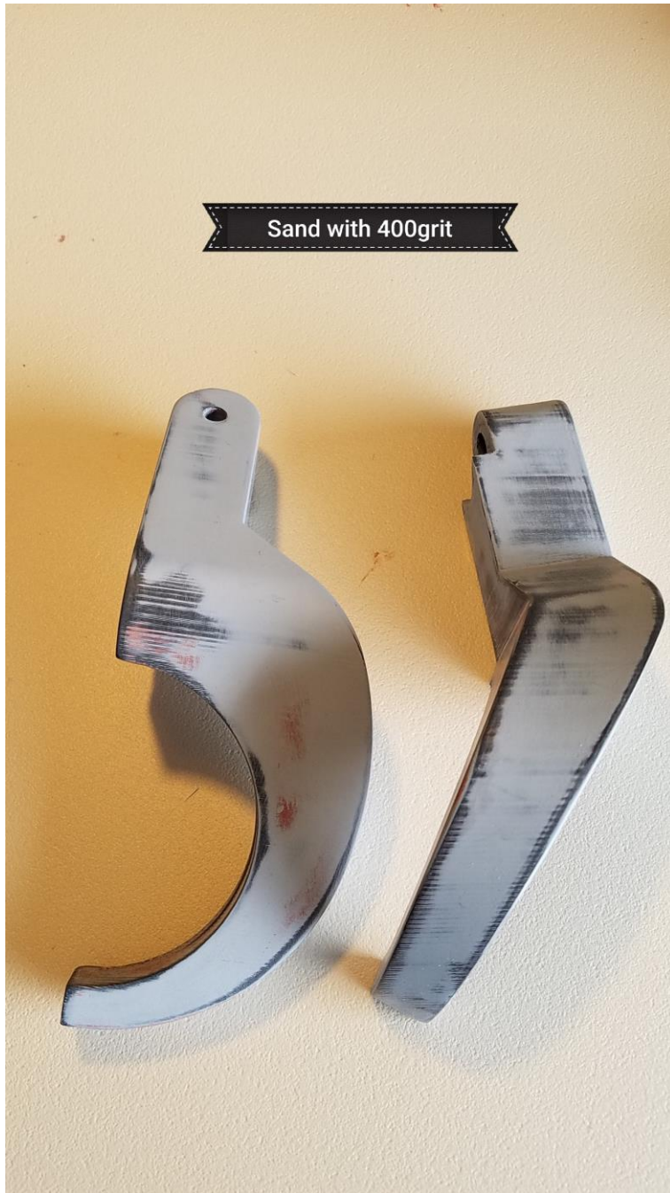
Pic 1n Using 400 grit. Lightly sand all surfaces under running water. After this step it will feel very smooth to the touch. Don't worry if you sand down to the black in spots.
