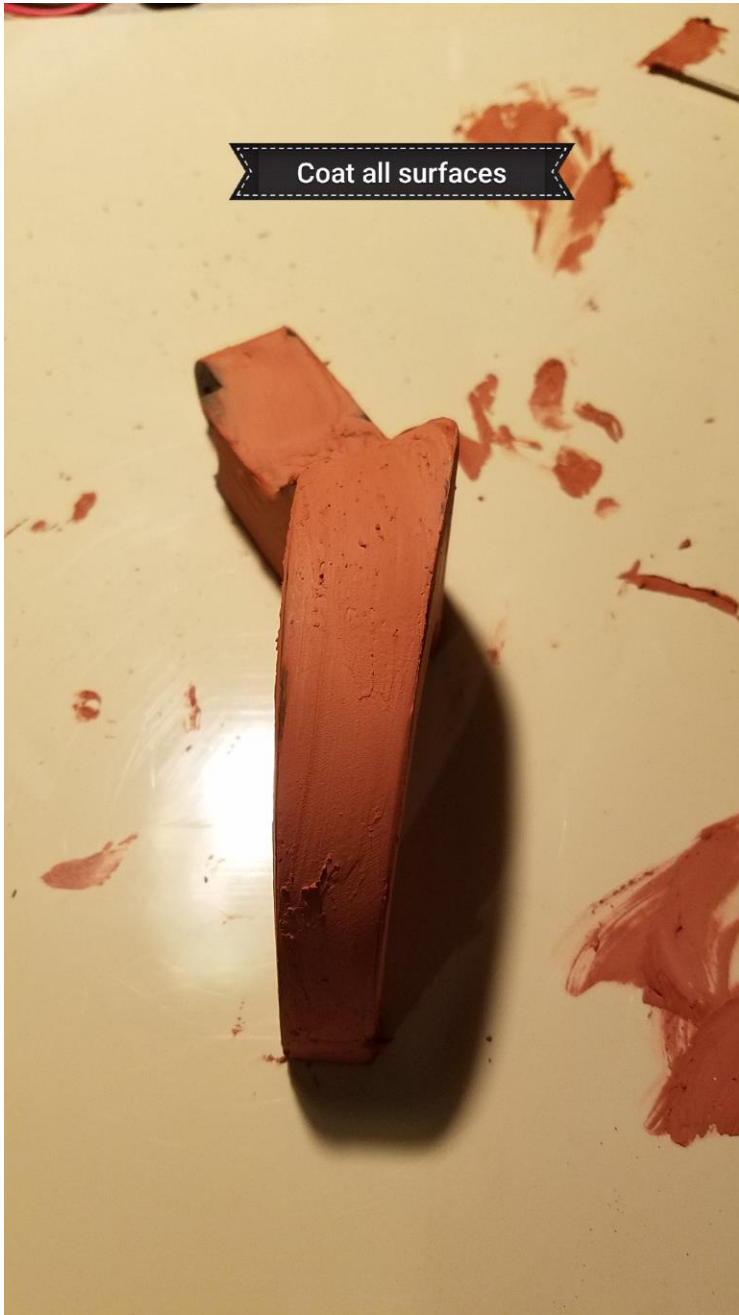
Pic 1j Smear Bondo glazing putty on all surfaces and let dry for at least an hour or two.
